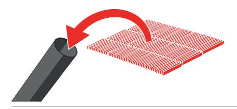
Place a pressure cap on top of the output pipe.
