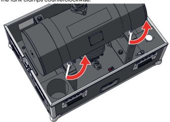
9 Set the tank with attached output pipe in an angle between 0 and 90 degrees.
