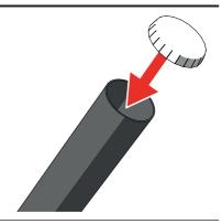
Secure the pressure cap to the output pipe with special pressure cap tape.
