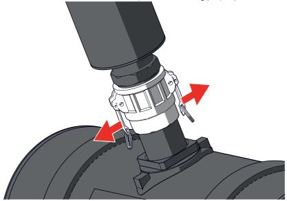
8 Turn the tank clamps counterclockwise.
