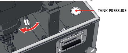
4 Pull the locking clamps downwards to unlock and rotate them upwards.
