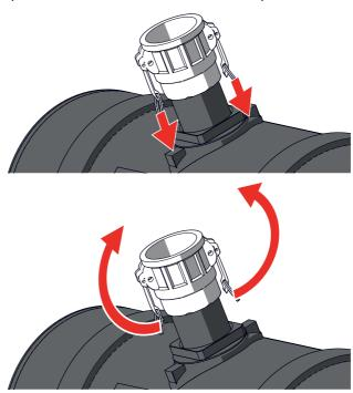
Place the output pipe in the coupling while holding the locking clamps upwards.
