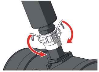
7 Pull the clamps outwards to check if the locking pins are properly locked in place.
