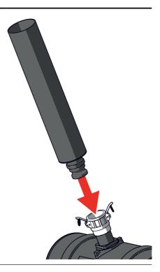
6 Lock the output pipe in place with the locking clamps.
