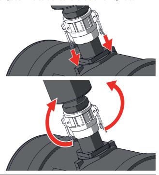
Remove the output pipe from the coupling.
