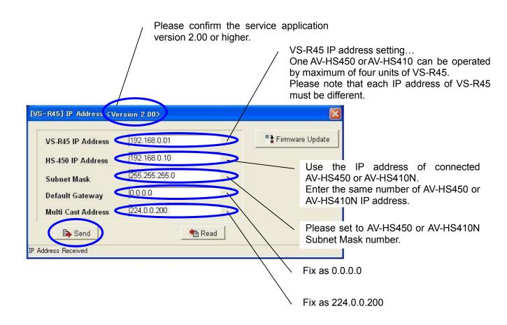
(8) "IP Address Set Complete" Screen appears on the status bar. This means that IP Address setting is completed. Click "x" button to close
