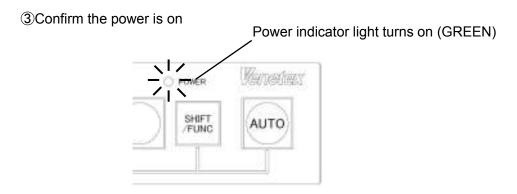
\*\*Operation begins when the VS-R45 is powered up by DC input.
